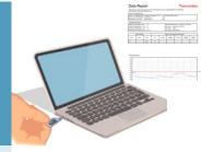
Plug Sensolabo® USB into a computer USB port. The PDF and CSV files are automatically **generated** and made available to your consignee.
