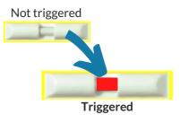
If your package has suffered a shock over the g force threshold, the tube in the middle of the indicator will irreversibly turn red.
